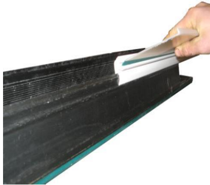
Figure 24 – sliding valve on to a Comfort Slat Mat
